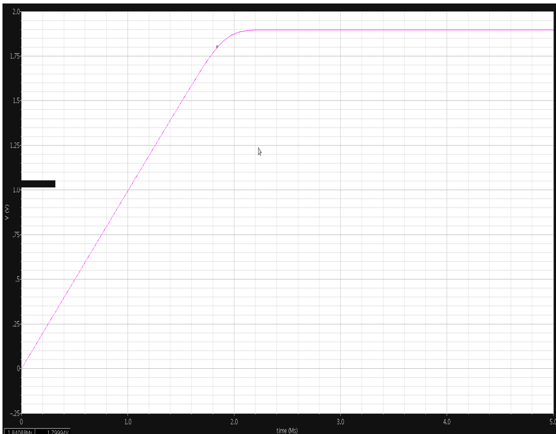
Figure 1.6. Time domain response of Three diode ItoV Converter with 100nA input current and 100mF capacitor across it.
