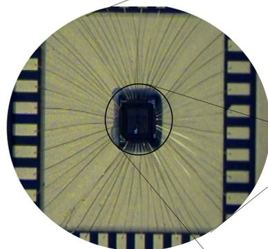
Photograph of silicon chip. Gold wire connections are visible and measure 60 x 60 μm.
