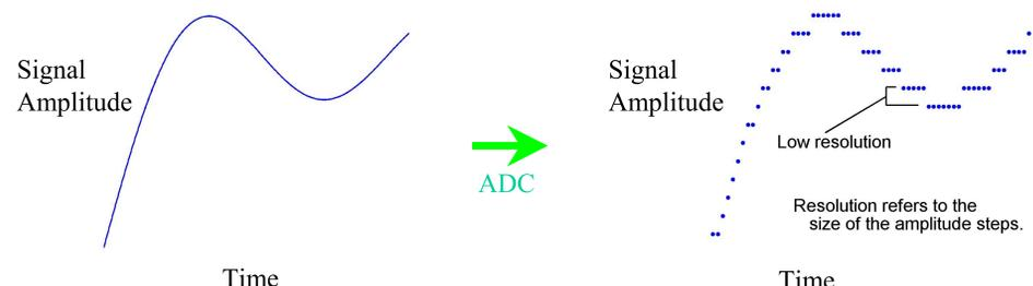
Analog signal from real world is defined at all points in time and amplitude.
