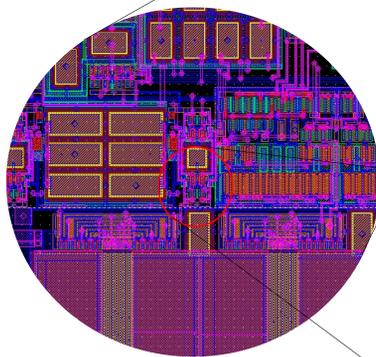
Highest magnification shows an individual transistor with a gate that measures 0.6 x 3 μm.
