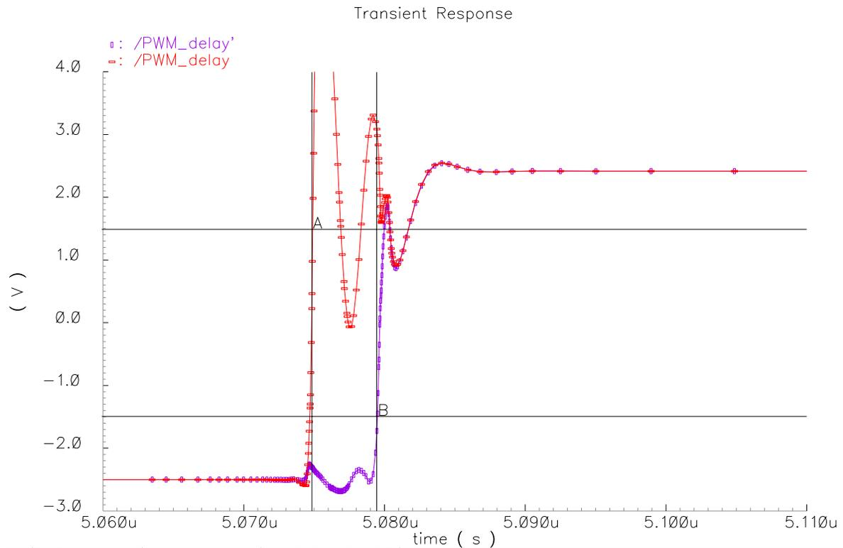
**Figure 3.14 – H-Bridge Driver Rising Edge Delay Waveform**
