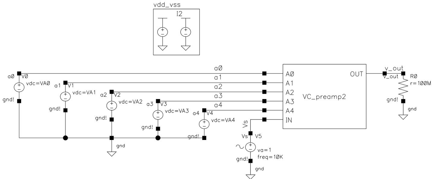
**Figure 3.9 – Volume Control Preamplifier Test Circuit**
