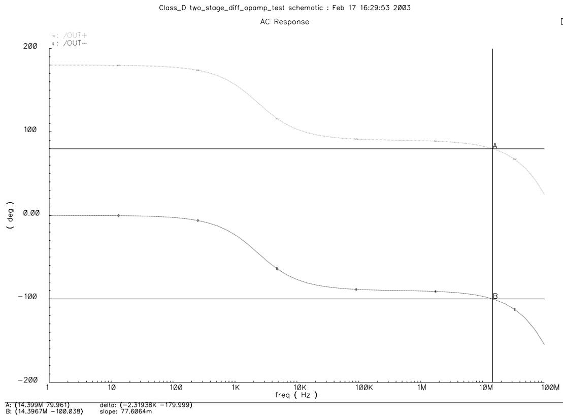
**Figure 3.2 – Fully Differential Operational Amplifier AC Response**
