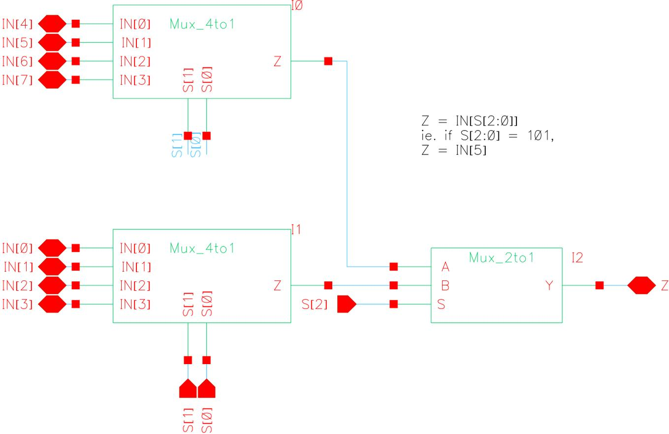
Figure A.8 – 8 to 1 Multiplexer Schematic
