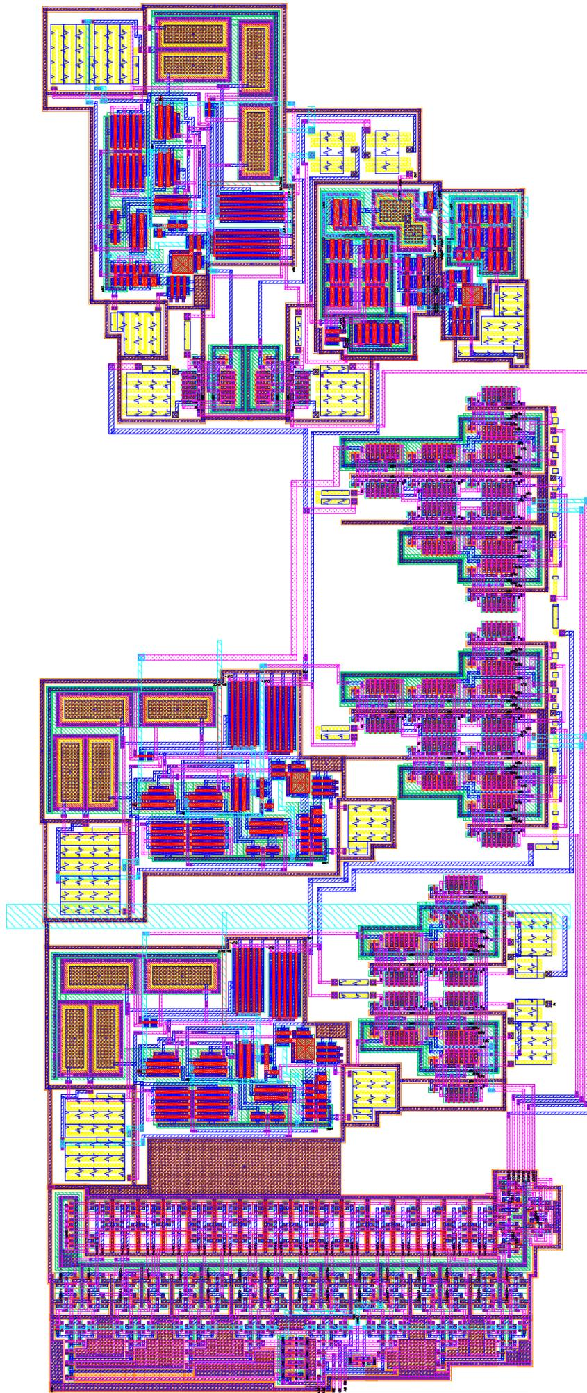
Figure B.8 -- Volume Control Preamp Layout
