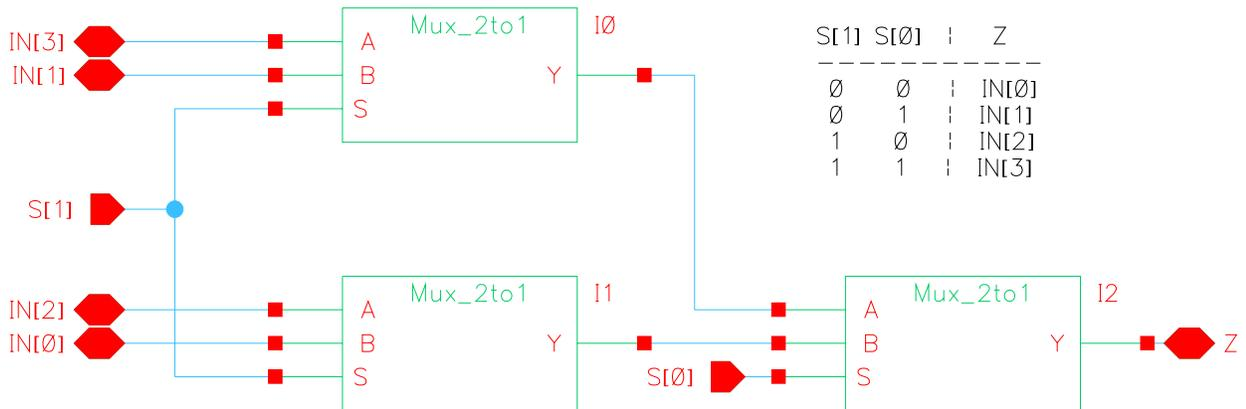
**Figure A.7 – 4 to 1 Multiplexer Schematic**
