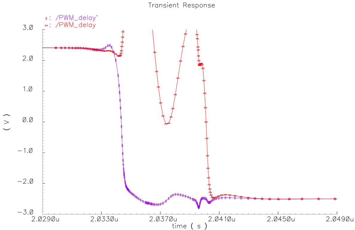
**Figure 3.13 – H-Bridge Driver Falling Edge Delay Waveform**
