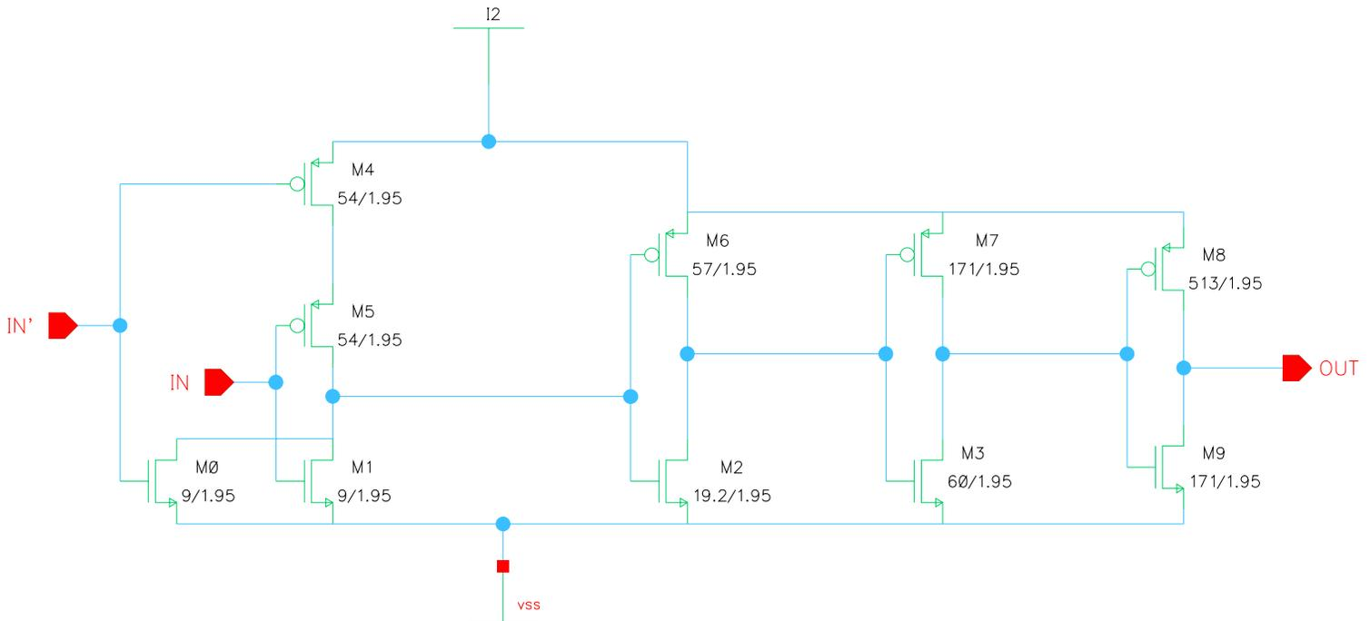
**Figure 2.13 – H-Bridge Driver Schematic**
