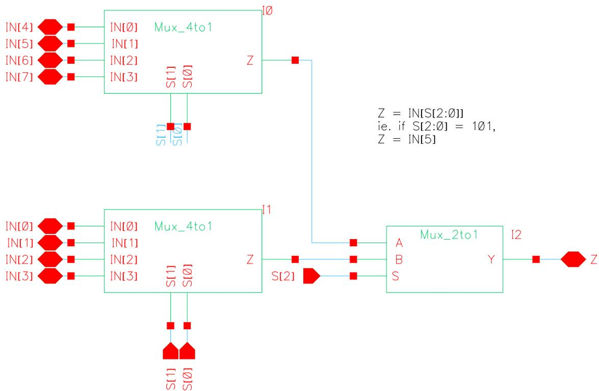
**Figure 2.4 – 8 to 1 Multiplexer Schematic**
