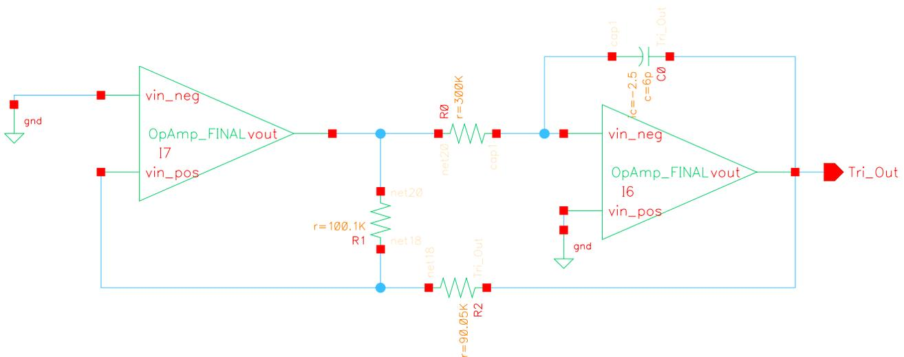
Figure 2.11 – Bi-Stable Oscillator Schematic
