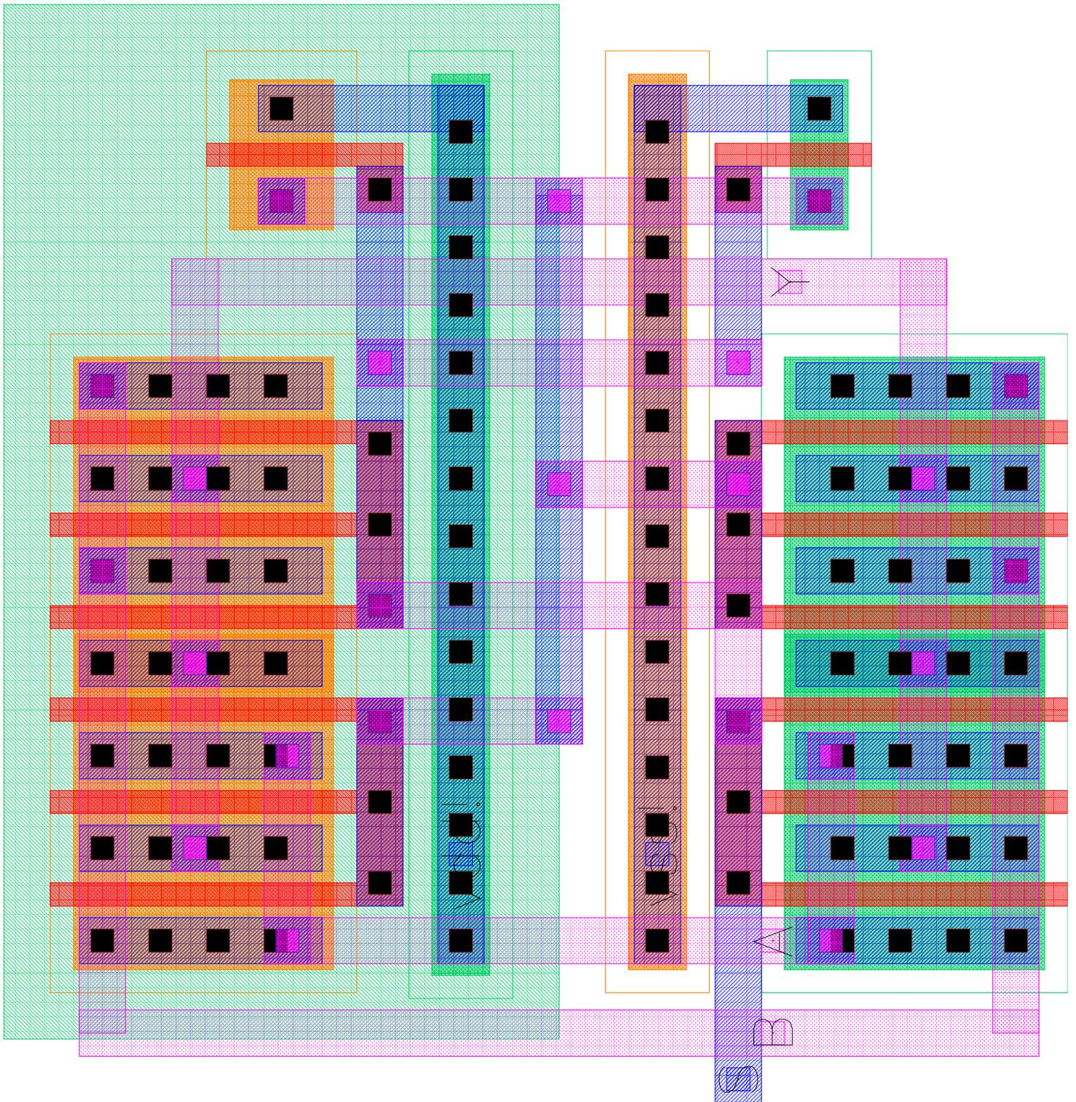
Figure B.3 -- 2 to 1 Multiplexer Layout
