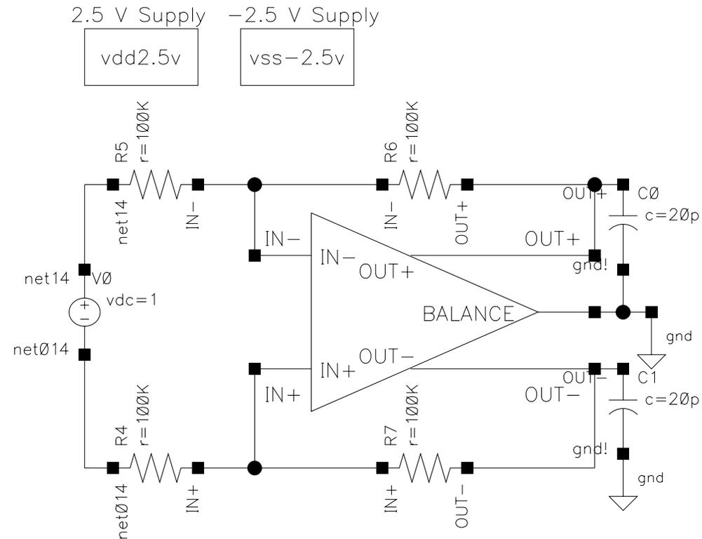
**Figure 3.3 – Fully Differential Operational Amplifier DC Test Circuit**
