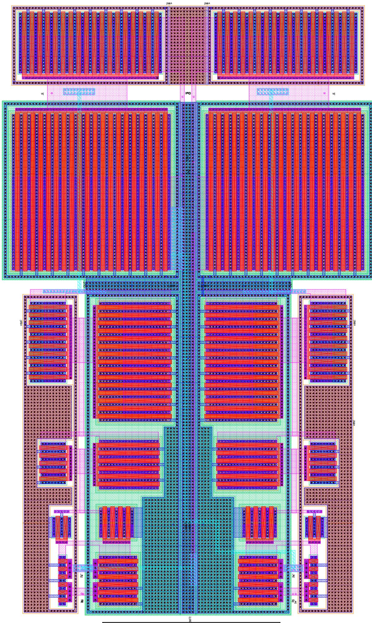
Figure B.11 -- H-Bridge Delay Layout
