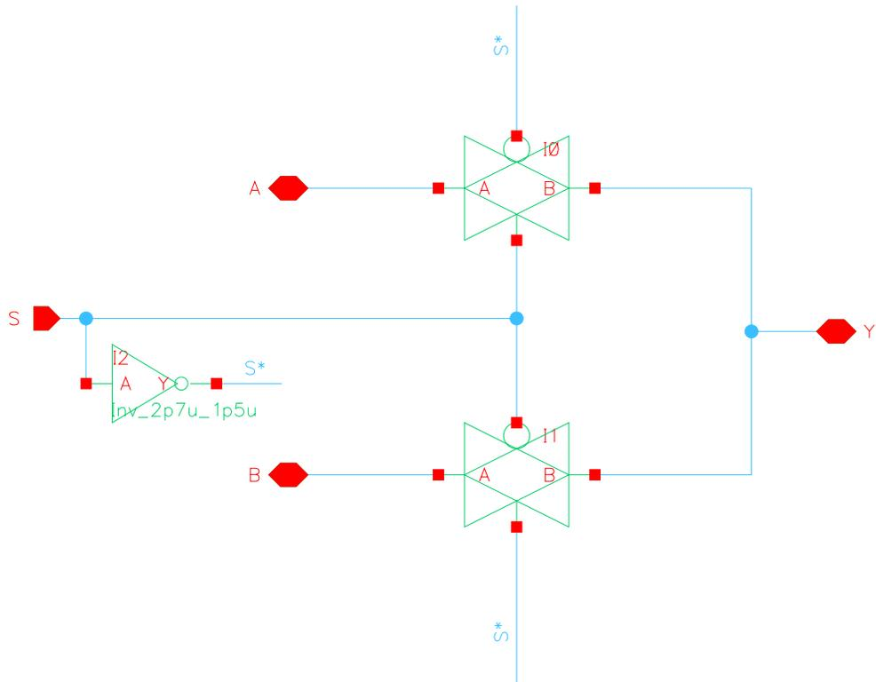
**Figure A.6 – 2 to 1 Multiplexer Schematic**
