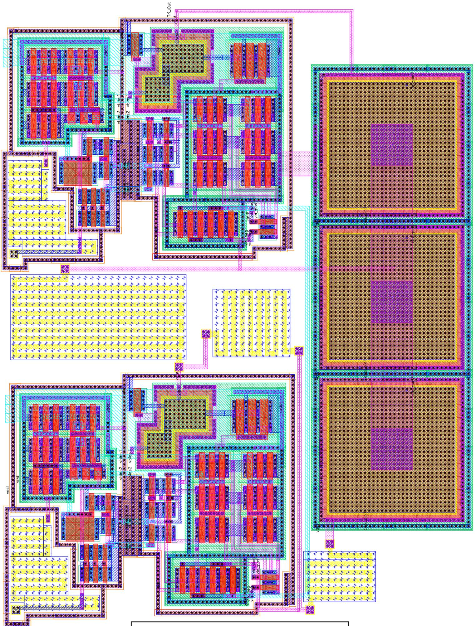
Figure B.9 -- Triangle Wave Generator Layout
