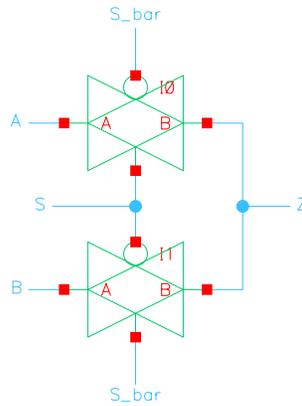
**Figure 2.2 – Transmission Gate Schematic**
