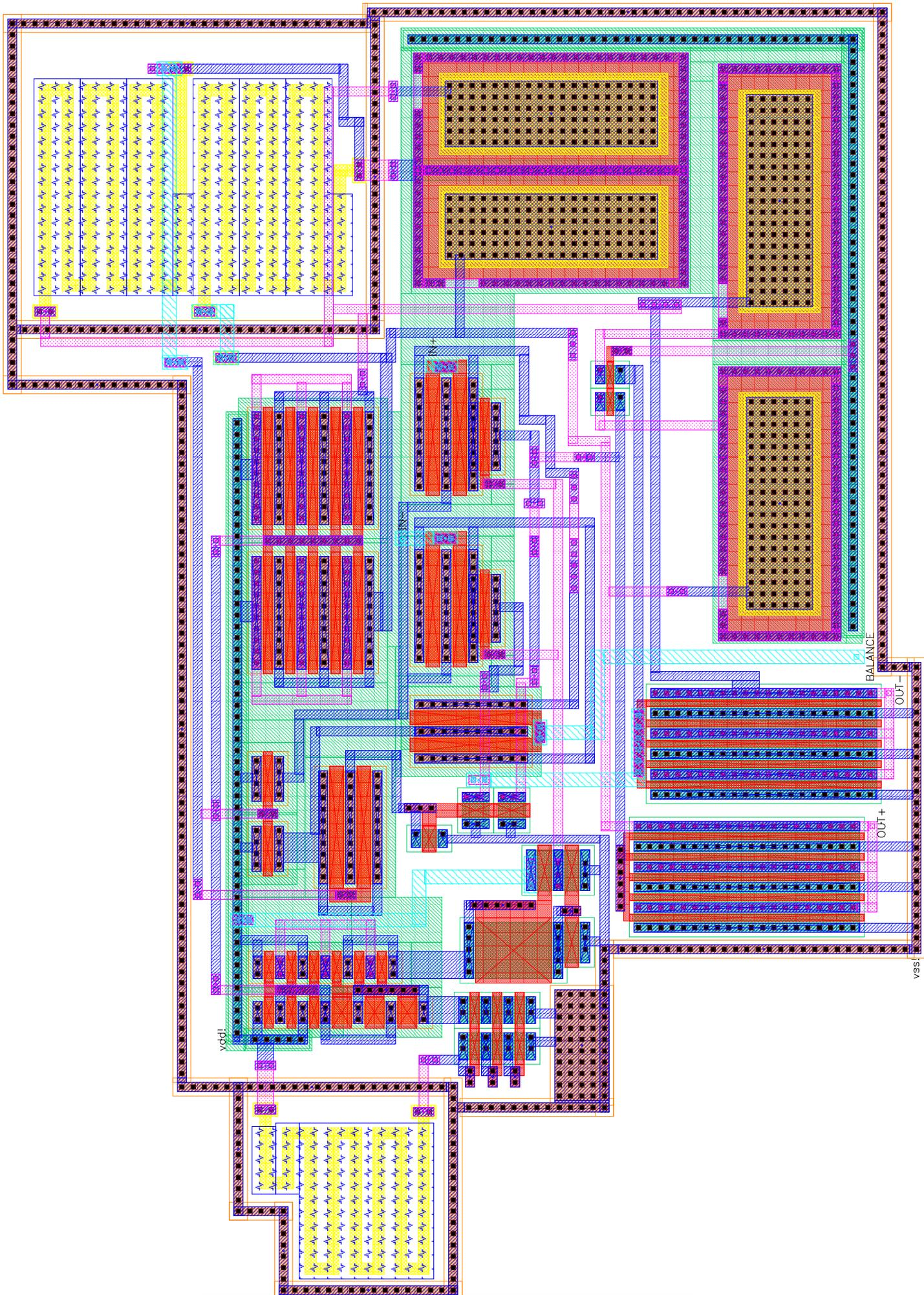
Figure B.1 -- Two Stage Differential Op-amp Layout
