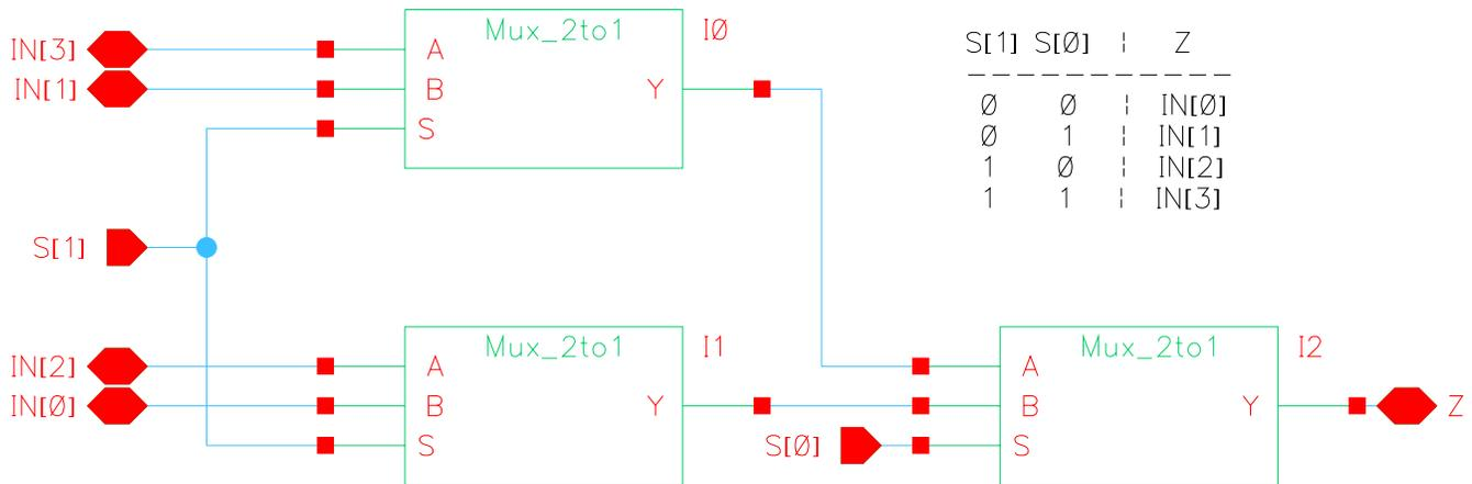
**Figure 2.3 – 4 to 1 Multiplexer Schematic**
