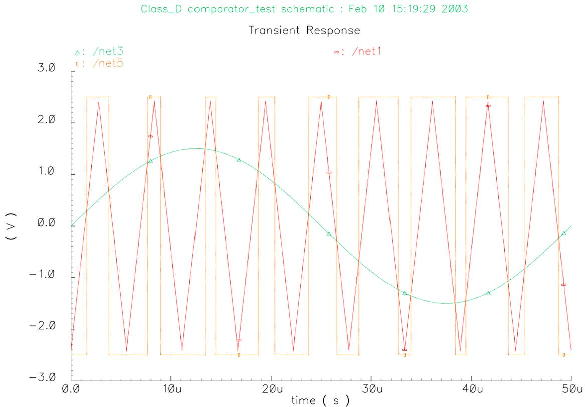
**Figure 3.12 – Comparator (PWM) Test Waveform**
