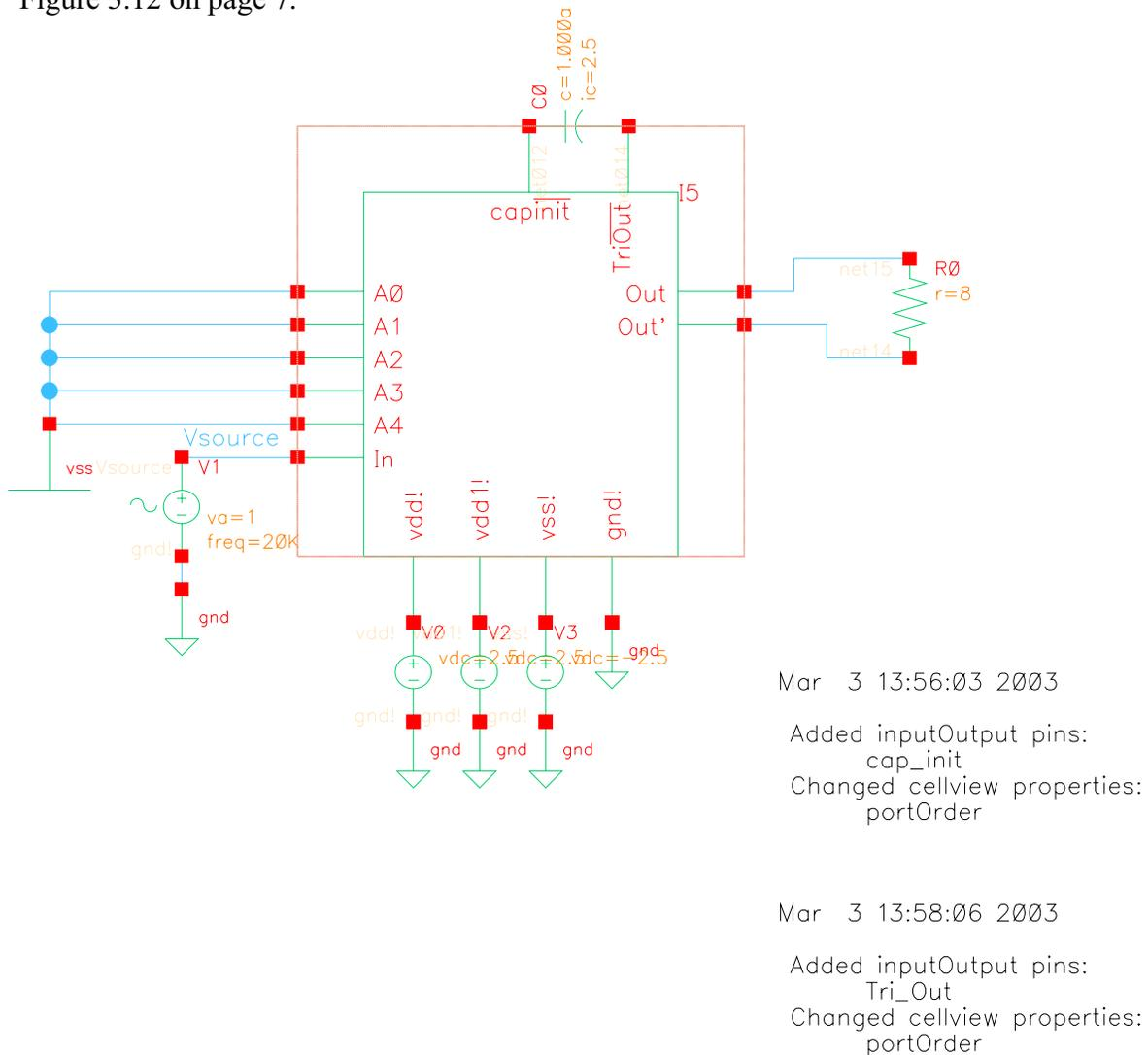
**Figure 5.1 – Top-Level Simulation Circuit with Parasitics**
