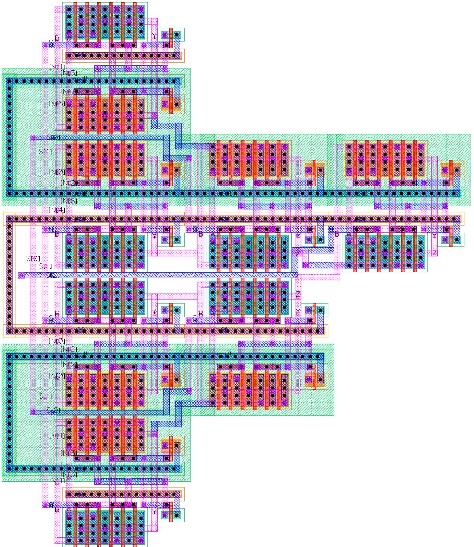
Figure B.5 -- 8 to 1 Multiplexer Layout
