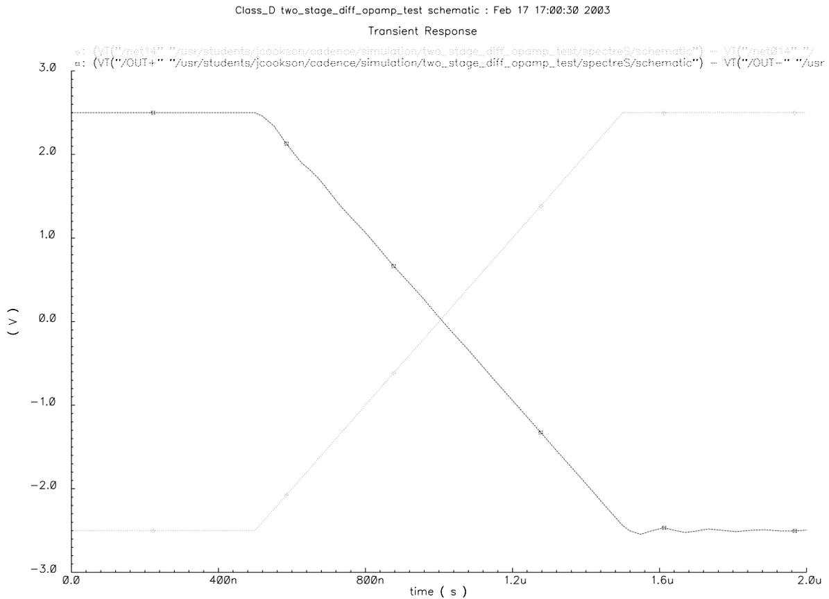
**Figure 3.6 – Fully Differential Operational Amplifier Transient Response**
