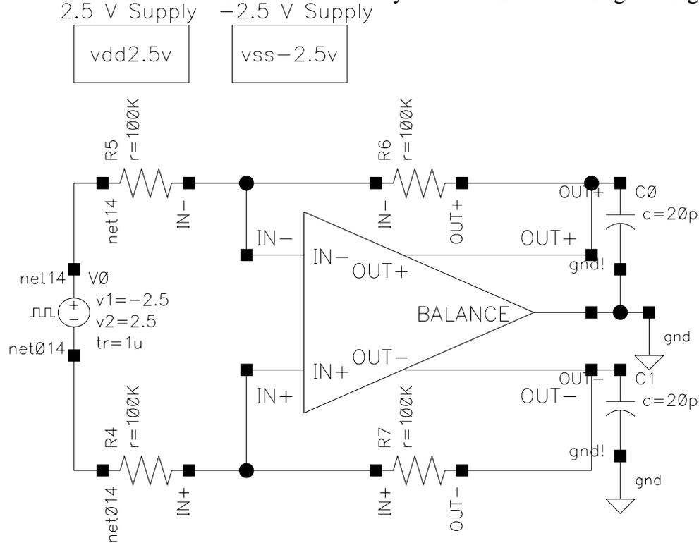
**Figure 3.5 – Fully Differential Operational Amplifier Transient Test Circuit**
