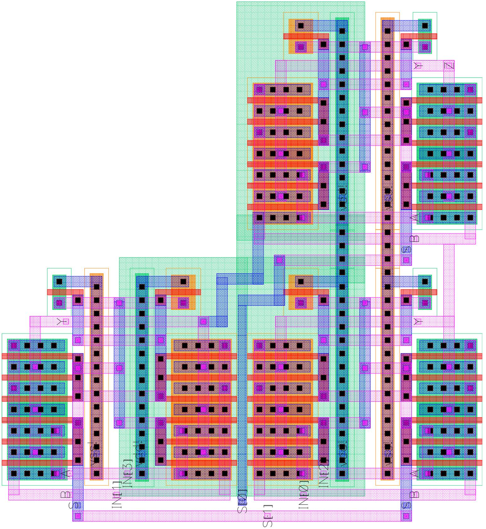
Figure B.4 -- 4 to 1 Multiplexer Layout
