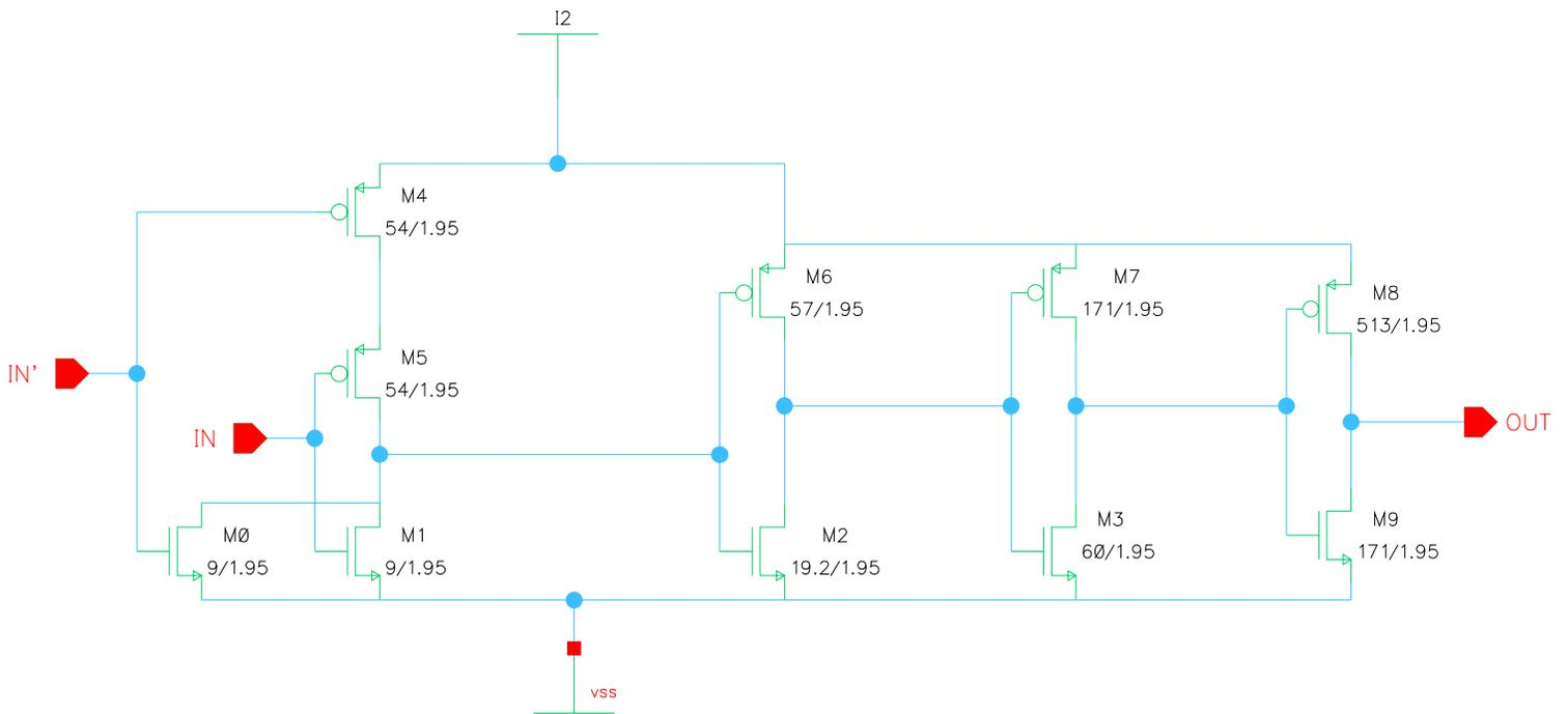
Figure A.15 – H-Bridge Delay Schematic
