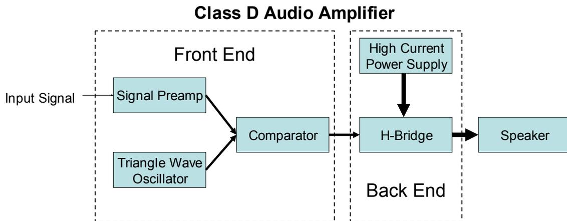
Figure 1.1 – Class-D Block Diagram
