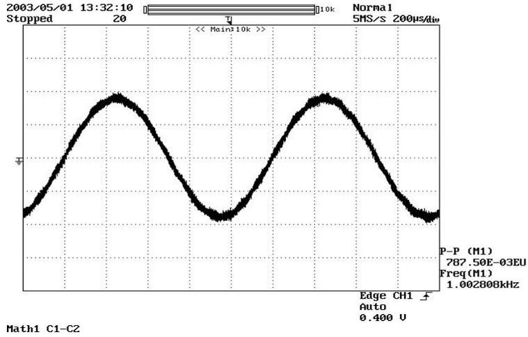
Figure 7.9: Design A Non-inverting Op-amp Test - Differential Output Measurement
