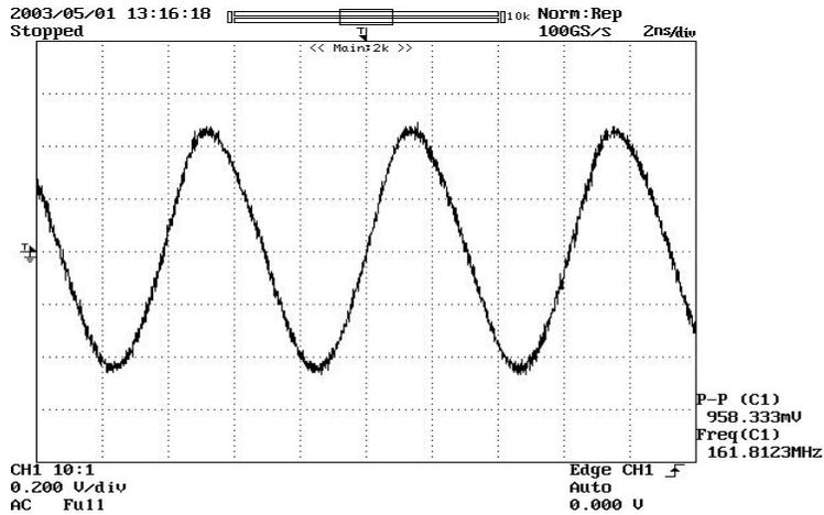
Figure 7.12: Ring Oscillator Output - Chip #1
