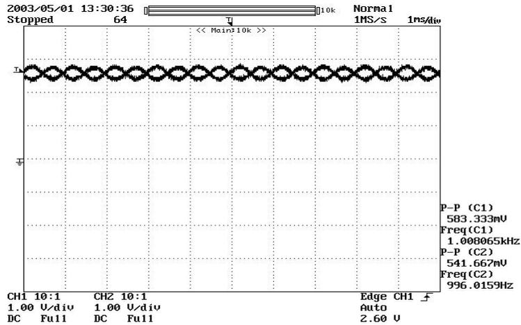
Figure 7.8: Design A Non-inverting Op-amp Test - Output Voltages
