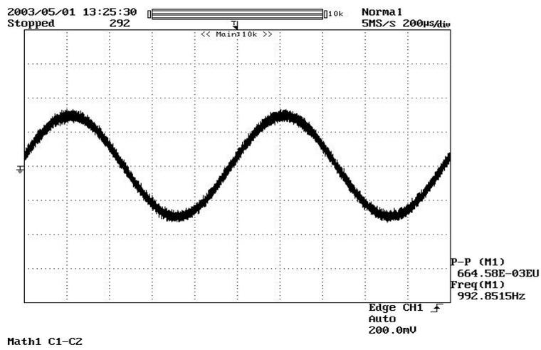
Figure 7.11: Design B Non-inverting Op-amp Test - Differential Output Measurement
