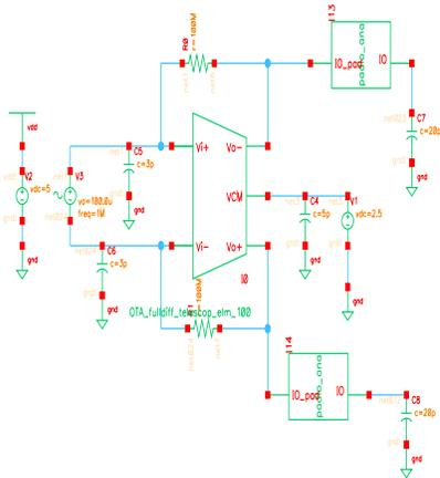
Figure 4.2: Test Circuit for Open-Loop Gain
