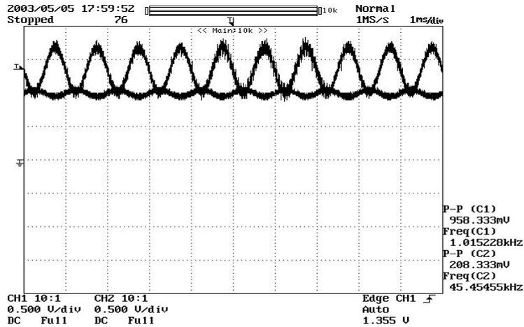
Figure 7.5: Typical Inverting Op-Amp Output (DC Coupled)
