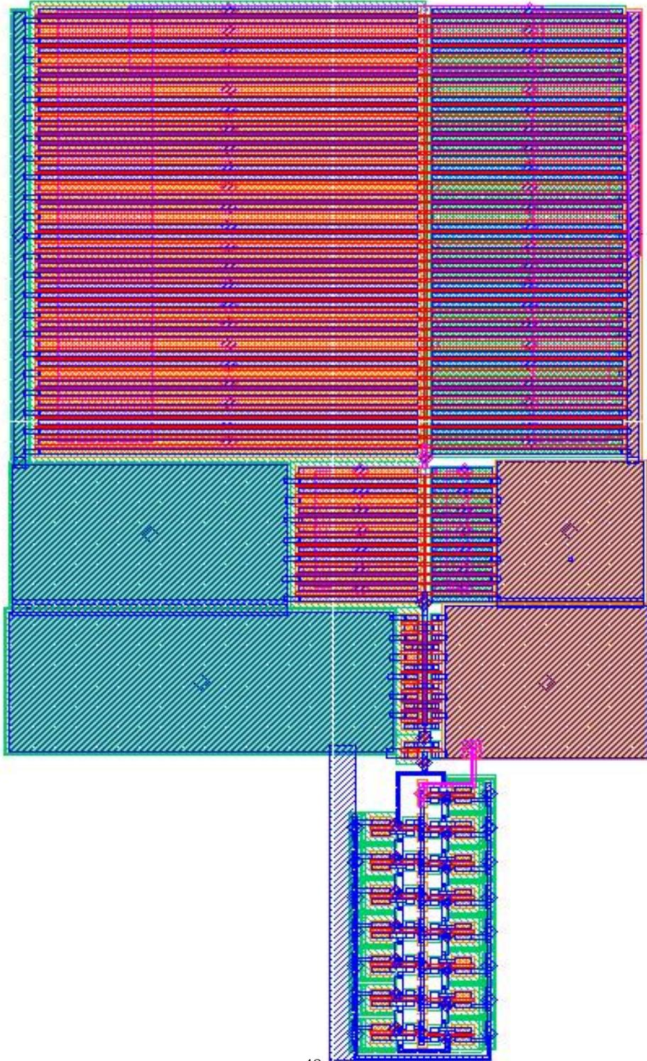
Figure B.5: 250MHz Ring Oscillator With Buffer
