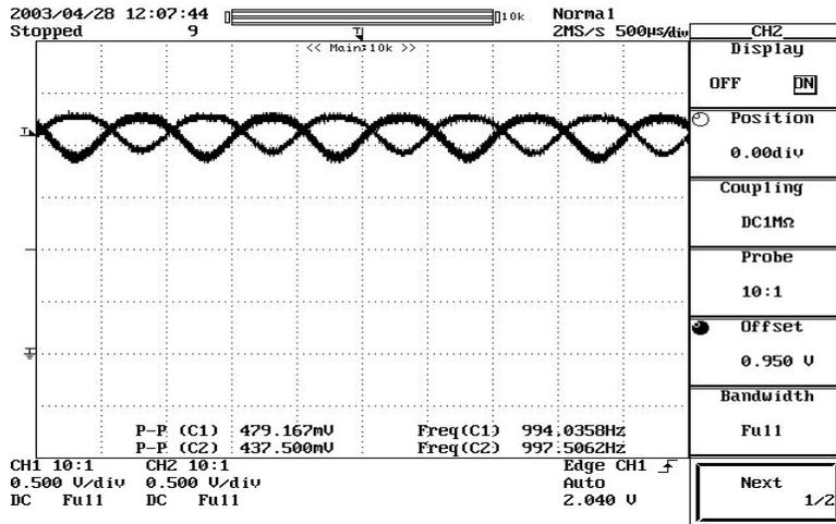
Figure 7.10: Design B Non-inverting Op-amp Test - Output Voltages
