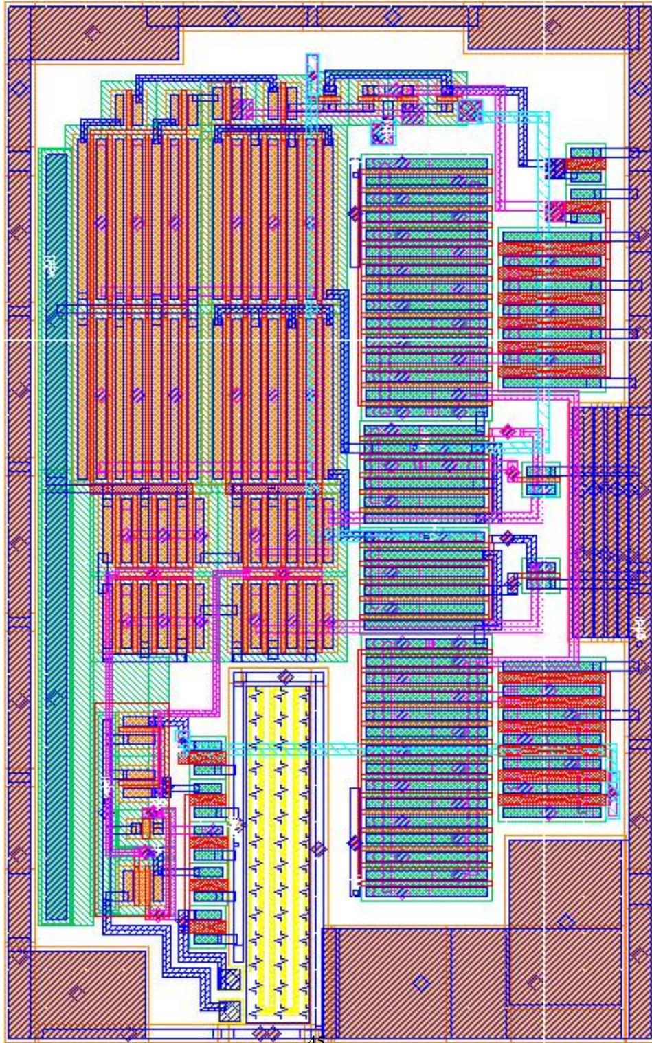
Figure B.2: Layout With Smaller CMFB Section (design A)
