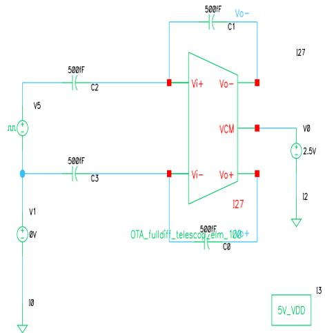
Figure 4.1: Test Circuit for Transient Response
