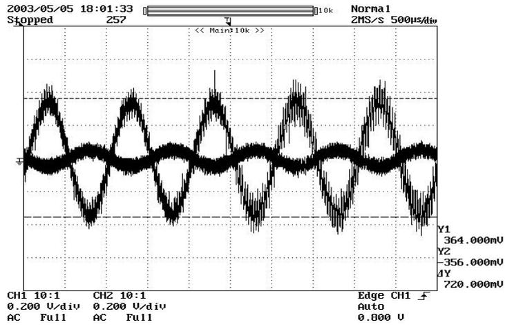
Figure 7.7: Design B Inverting Op-amp Test - Gain Measurement
