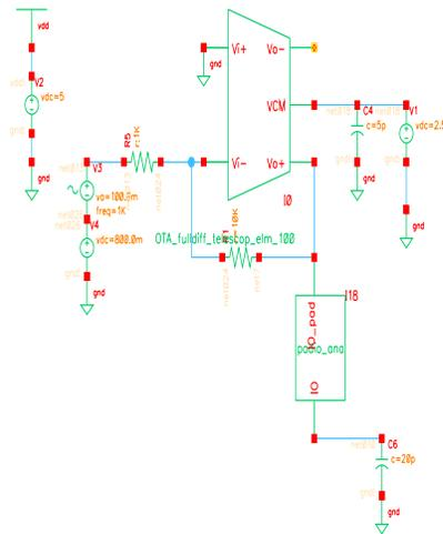
Figure 4.3: Test Circuit for Inverting Amplifier
