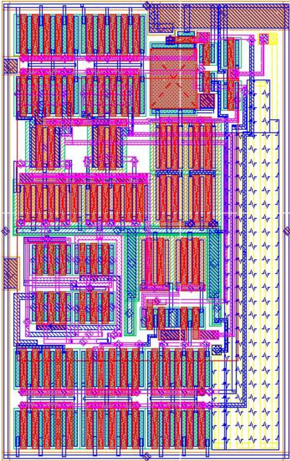
Figure B.4: Cascoded OTA Used In Previous ADC design
