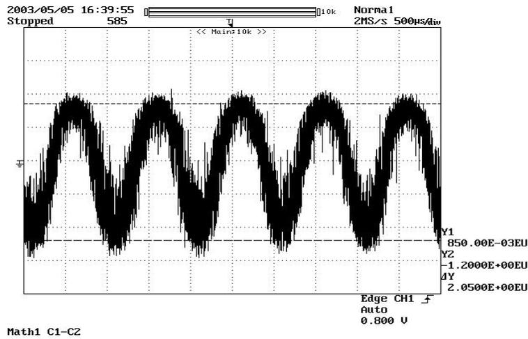
Figure 7.1: Open Loop Gain Measurement - Design A
