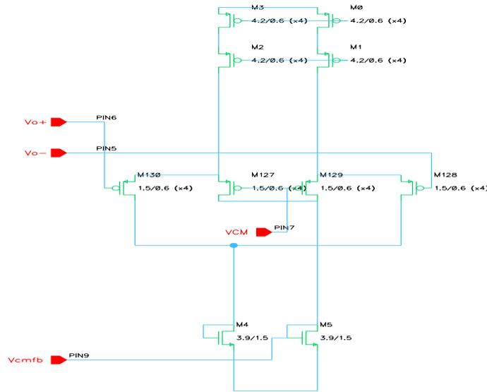
Figure 3.4: Common-Mode Feedback Circuit
