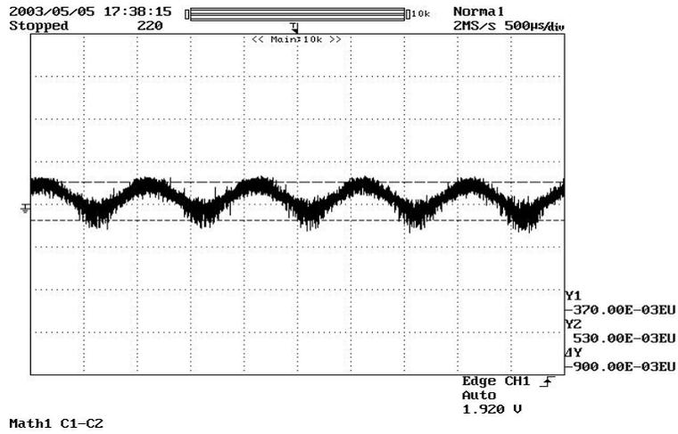
Figure 7.2: Open Loop Gain Measurement - Design B
