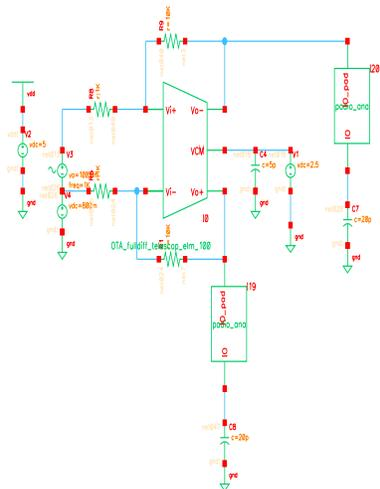
Figure 4.4: Test Circuit for Non-inverting Amplifier
