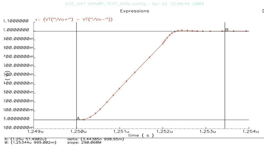
Figure 4.6: Settling Time Measurement for Rising Edge
