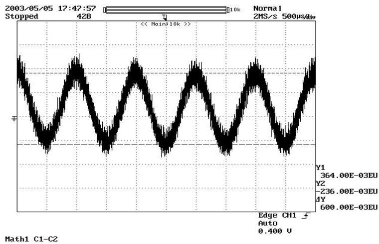
Figure 7.4: Open Loop Gain Measurement - Cascoded OTA
