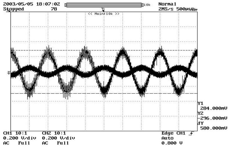
Figure 7.6: Design A Inverting Op-amp Test - Gain Measurement
