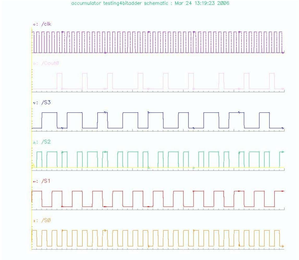
*Fig 17. Output waveform of 4 Bit Accumulator.*
