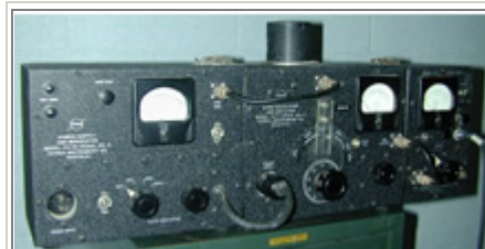
Power supply/modulator oscillator/amplifier
