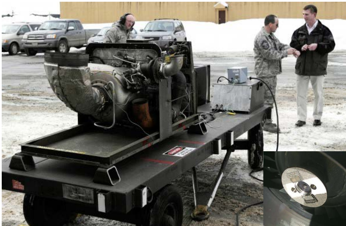
Jet engine equipped with state-of-the-art temperature sensor.
